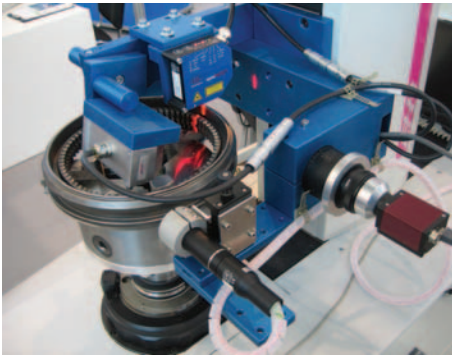
100% inspection using multiple Micro-Epsilon optical sensors
